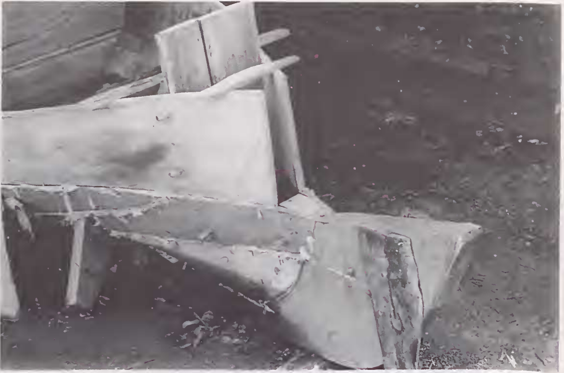
Fig. 21. Stern of perahu compreg under construction, the planking is in place and the aft frame or apron has been fitted but the sternpost is not yet fitted.
